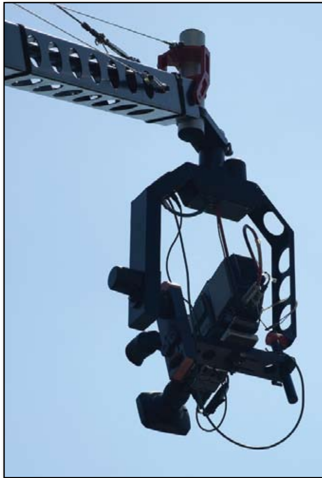
Figure 1: Wireless webcams for construction can transmit high-resolution photographs, PTZ photographs, or video.
